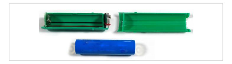
• Take out the battery part, battery bracket has two parts linked by connector. Open any one of them and take out the battery.
