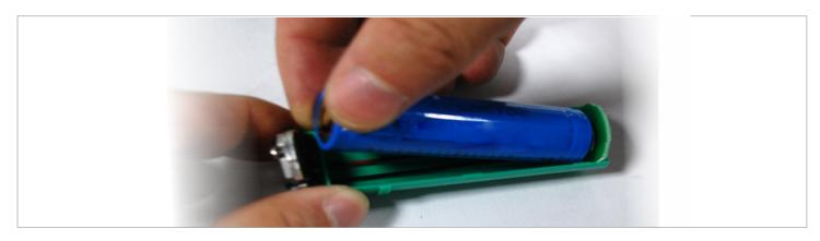
• Replace the battery, assemble the PCB board with spring and battery bracket firstly, and then put one side of battery into PCB board with spring tightly, after that press the battery into the battery bracket, cover the other part of battery bracket.
